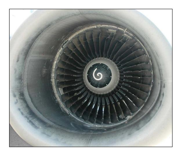
At the front side of the fan the air intake duct broke up at several places. There was a track of damage all around the duct following the counter clockwise rotation of the fan (pictures below).
