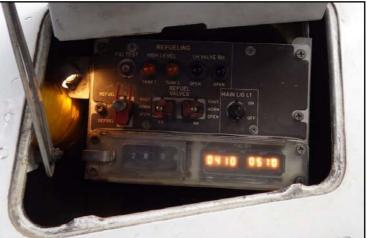
The fuel quantity indicator and the repeater were replaced with new units. The new indicators indicated the same values as presented above. The original indicators were reinstalled.
