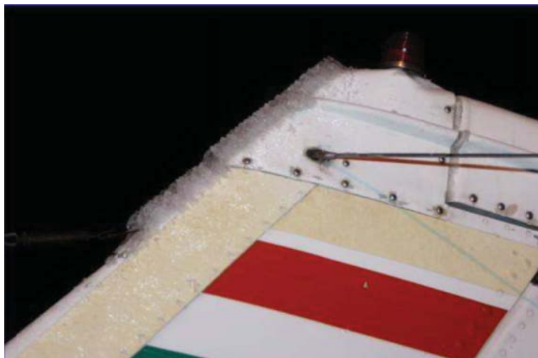
Ice on low radius of curvature aerofoils
