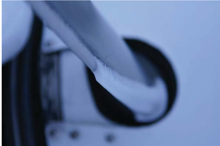
Ice on propeller blade
