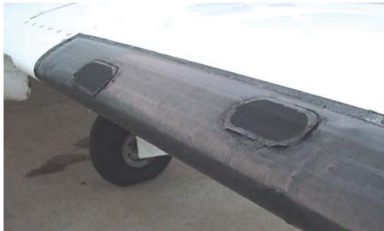
De-Icing Boot with Patch Repairs
