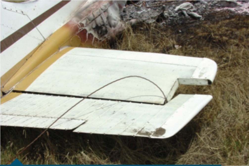
Section of the struck powerline caught in the horizontal stabiliser
