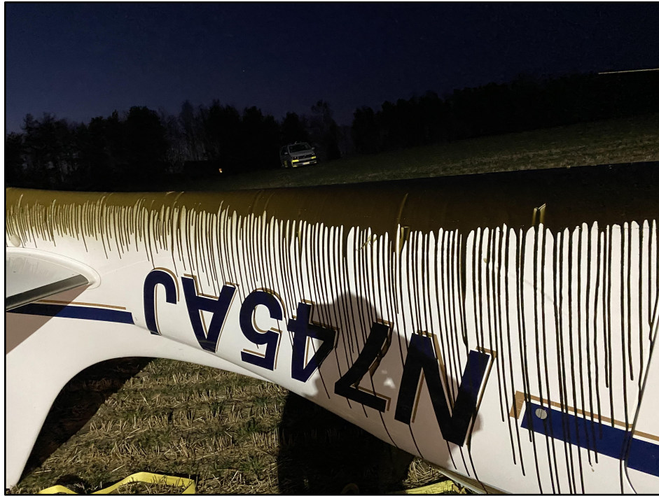
Photo 21. Engine oil on the underside of the aircraft fuselage.
