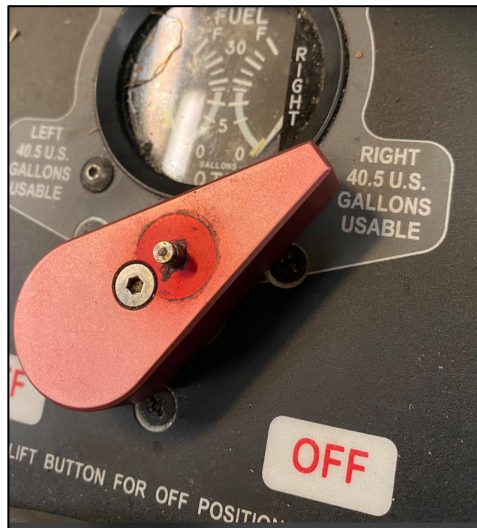
Photo 22. The release knob on top of the fuel selector handle was missing.
