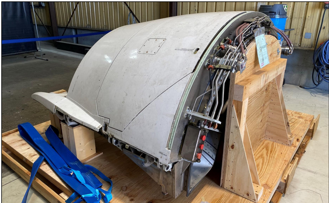
Figure 16. Engine #1 thrust reverser LH D-duct
