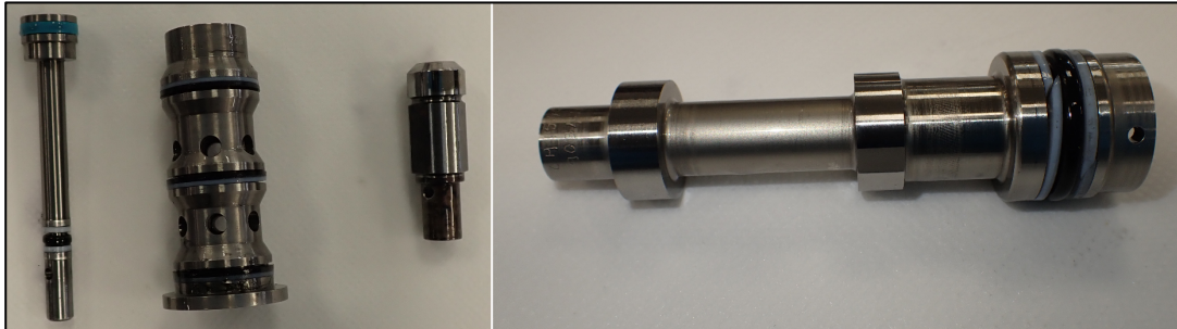
Figure 19. Isolation valve and associated parts shown left, and directional valve shown on the right
